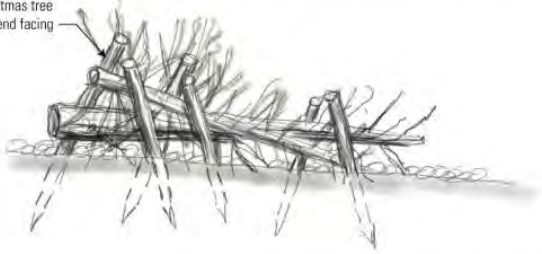
Figure 27 – Ideas for material substitutions with small root-wads and discarded/recycled Christmas trees or tops off of conifers. Smaller PALS like these can also be helpful to start with in streams and rivers with higher flow, to build something small and get it anchored, and then start piling on more material and pining it as necessary to produce something like found in the schematics.
